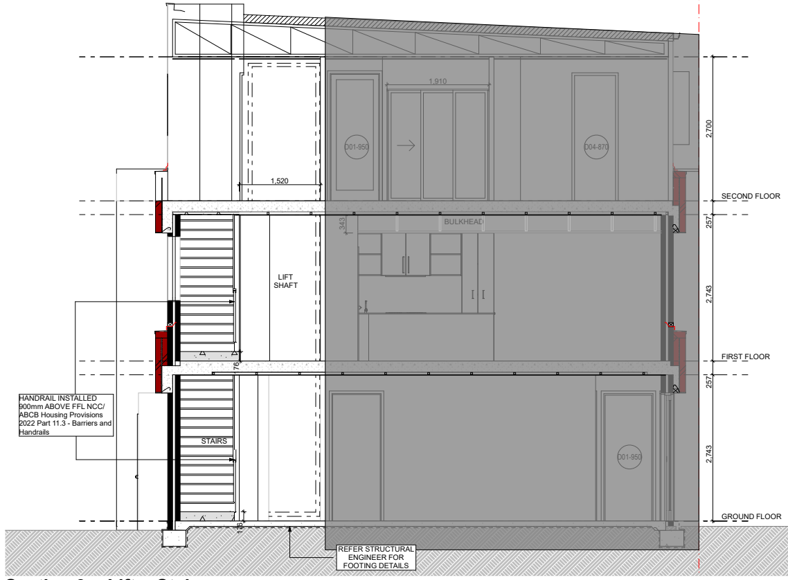
Section 3 - Lift + Stairs Scale 1:50
